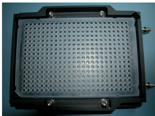
Figure 1. The micro-plate chuck (left). Its metal body is passed through coolant. The cooling effect can be seen in the right diagram.
